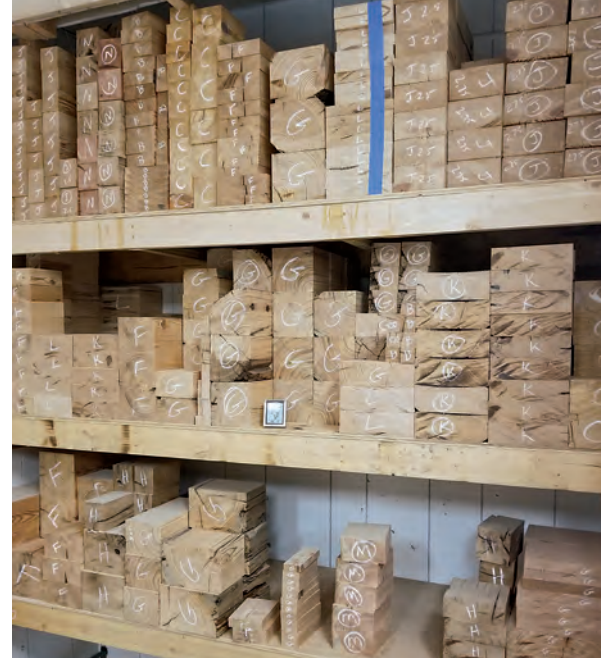
Most of the table's 1,008 pieces were first milled into 6"-long blanks, then labeled with chalk and carefully cataloged prior to assembly.
